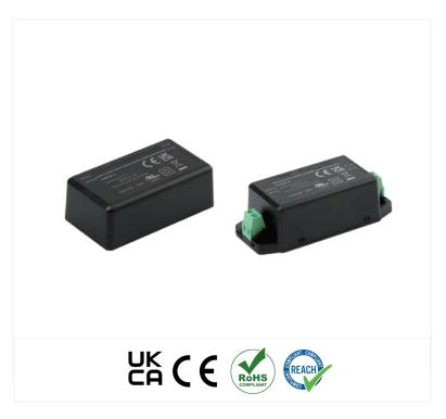
The 56YMR45-xx Series is a consistent and reliable 45W Encapsulated AC/DC PCB Mount Power Supply. Designed for use in applications such as commercial AV, broadcasting and control panels. This series is supplied with a Pin Connection or Screw Terminal input connection and supports input voltages of 85~305V AC 47-63Hz.
